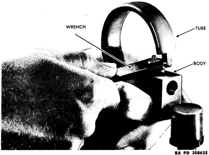
**Figure 37 – Removing Upper Valve Guide, Using
