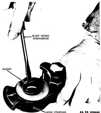
Figure 140 – Installing Hose Coupling Gasket (Final Operation)
