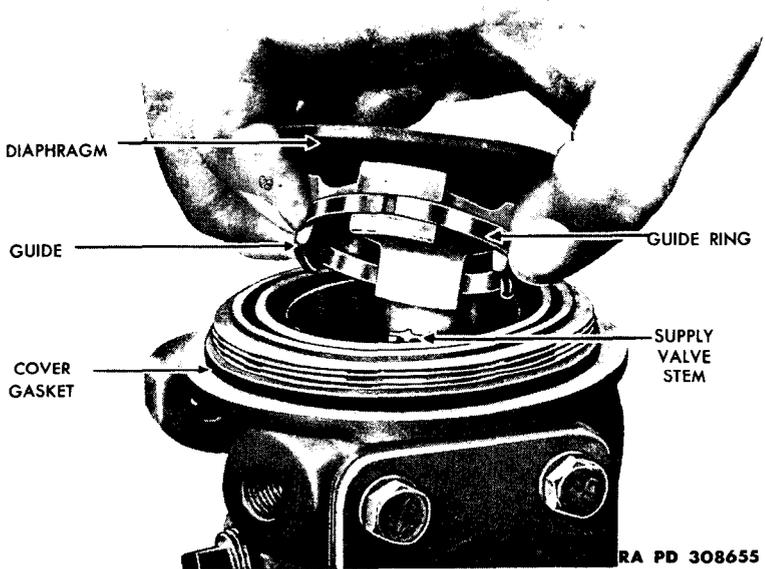
**Figure 92 – Installing Diaphragm and Guide Assembly**
