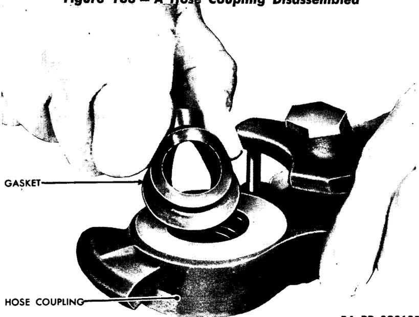
**Figure 139 – Installing Hose Coupling Gasket (First Operation)**
