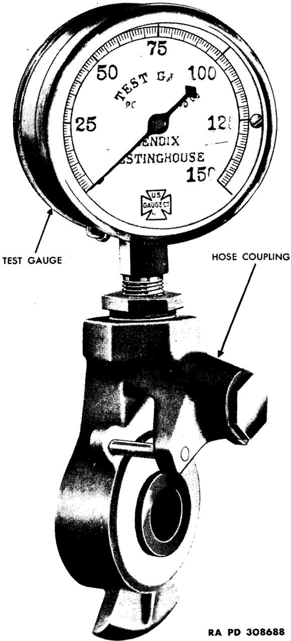
Figure 156 — A Test Gauge
