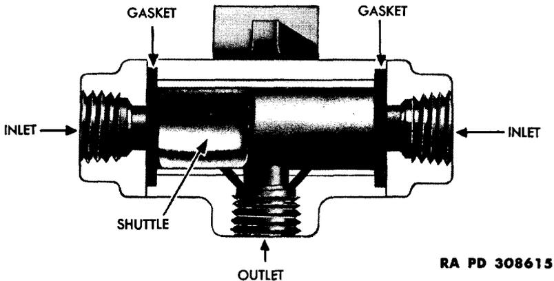
**Figure 119 – Sectional View of Double Check Valve**
