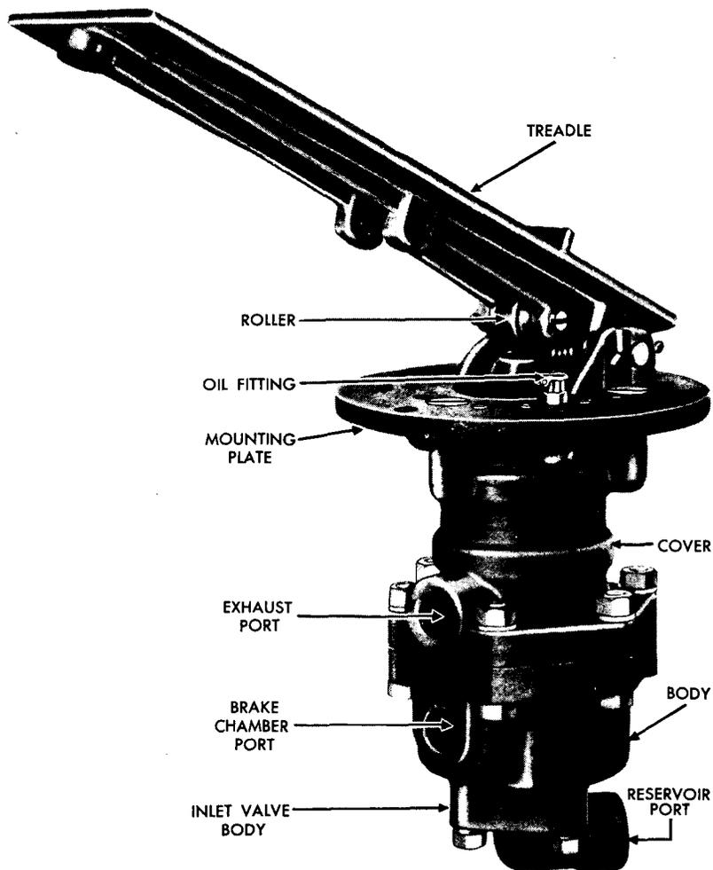
**Figure 68 — Type-D Brake Valve**
