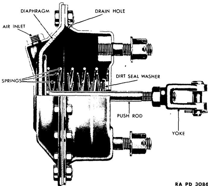
Figure 102 — Sectional View of a Stud-type Brake Chamber
