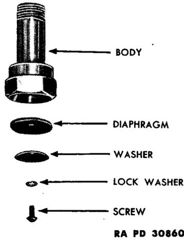
**Figure 122 – Exhaust Check Valve Disassembled**
