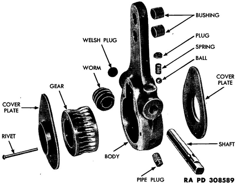
**Figure 111 — A Type-K Slack Adjuster Disassembled**
