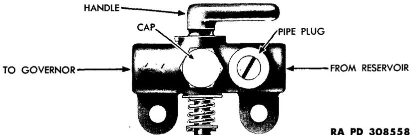
**Figure 157 - Air Supply Valve**
