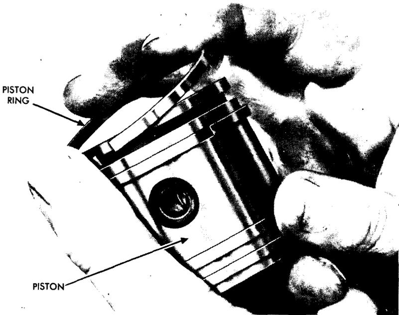
**Figure 30 – Installing Piston Rings**
