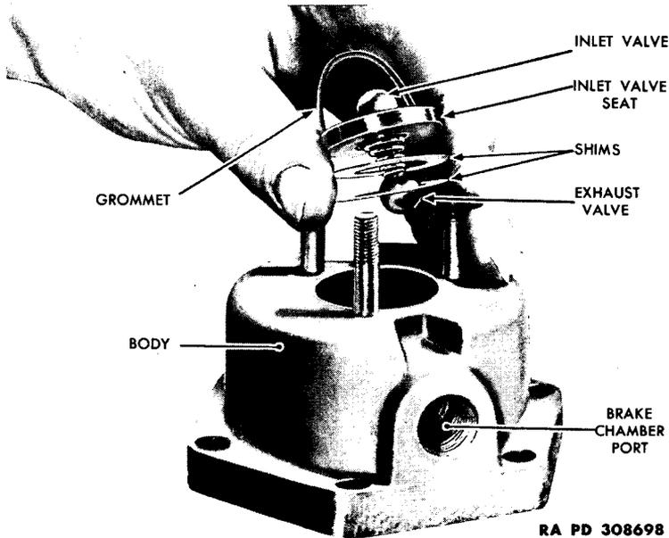
**Figure 73 — Removing Inlet and Exhaust Valve Assembly**
