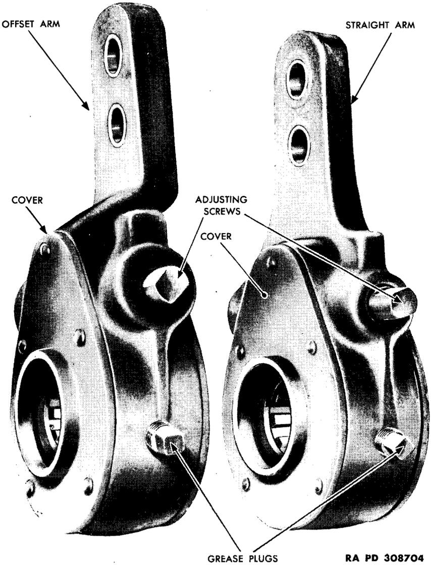
Figure 109 – Type-K Slack Adjusters with Straight and Offset Arms
