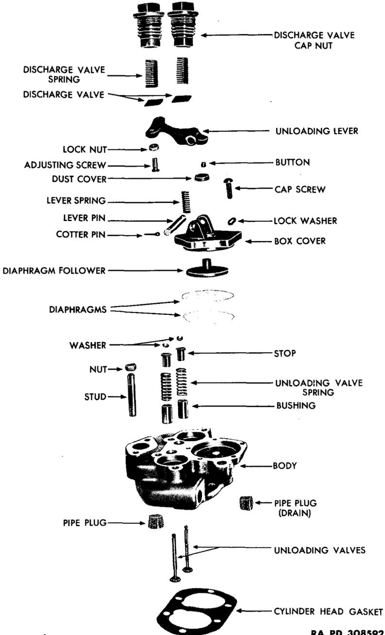
**Figure 13 — A Two-cylinder Compressor Cylinder Head Disassembled**
