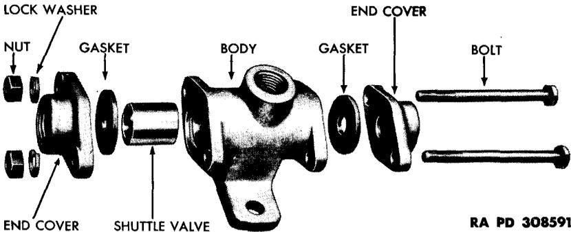
**Figure 120 – Double Check Valve Disassembled**
