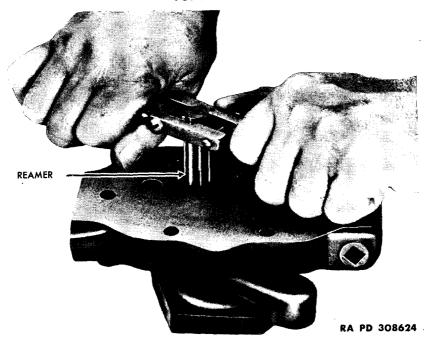
Figure 22 – Reaming Unloading Valve Seats, Using Reamer 41-R-2309
