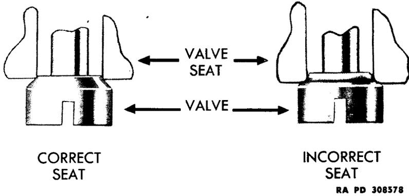
Figure 57 — Correct and Incorrect Valve Seats
