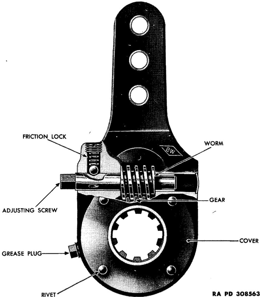
**Figure 110 — Sectional View of a Type-K Slack Adjuster**
