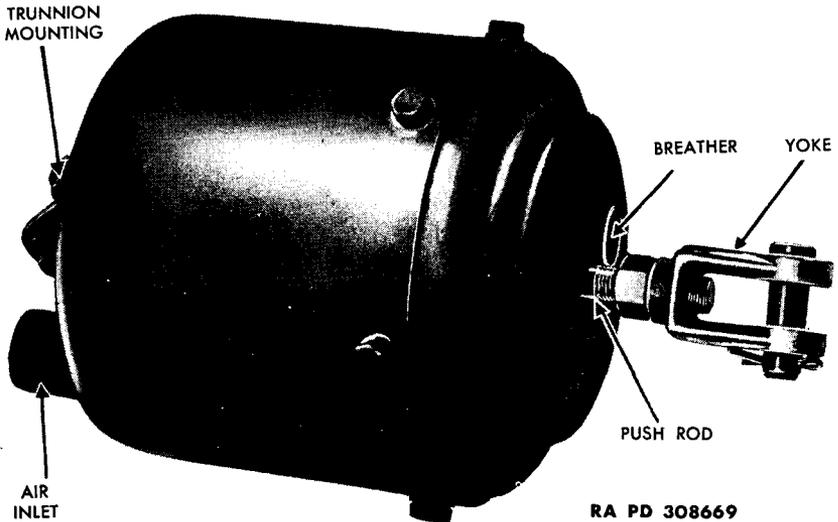
**Figure 106 – A 6-inch x 3-inch Brake Cylinder**
