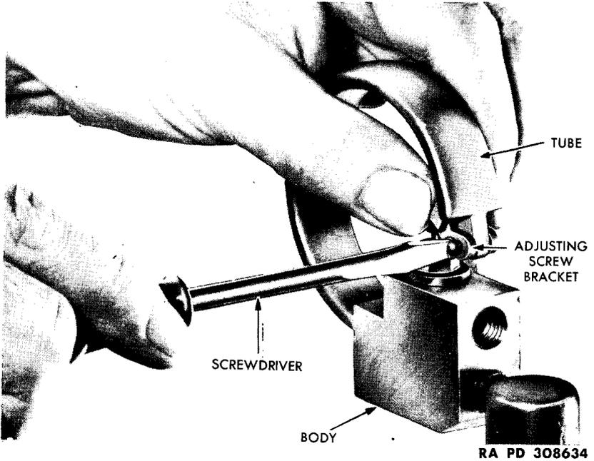
**Figure 36 – Removing Adjusting Screw Bracket**
