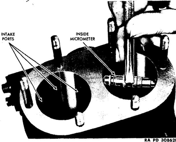
**Figure 19 — Measuring Cylinder Bore Diameters, Using Tool 41-C-304**
