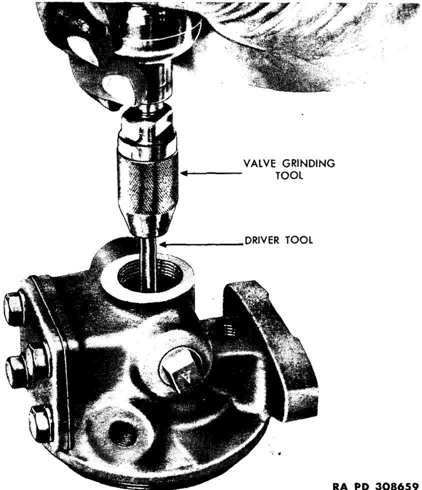
**Figure 88 – Grinding Supply Valve, Using Tools 41-T-3381-15
