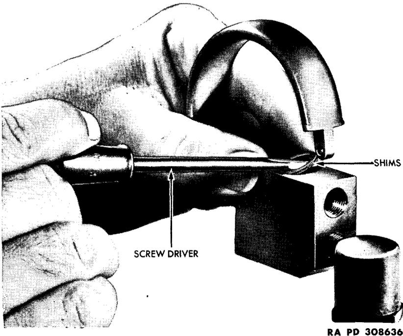
**Figure 38 – Removing Shims**
