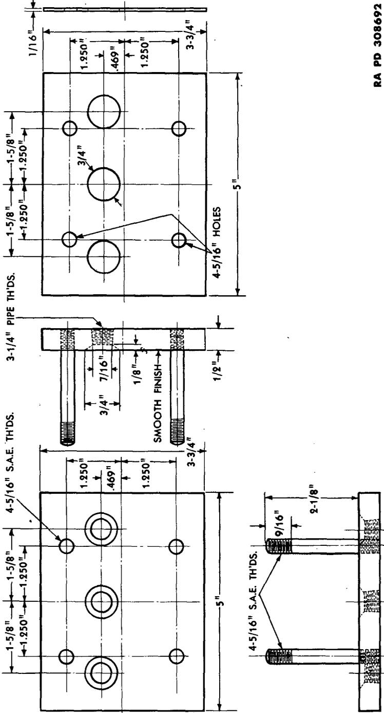
Figure 175 -- Line Drawing of Fixture for Testing Unloading Valves of Three-cylinder Compressors
