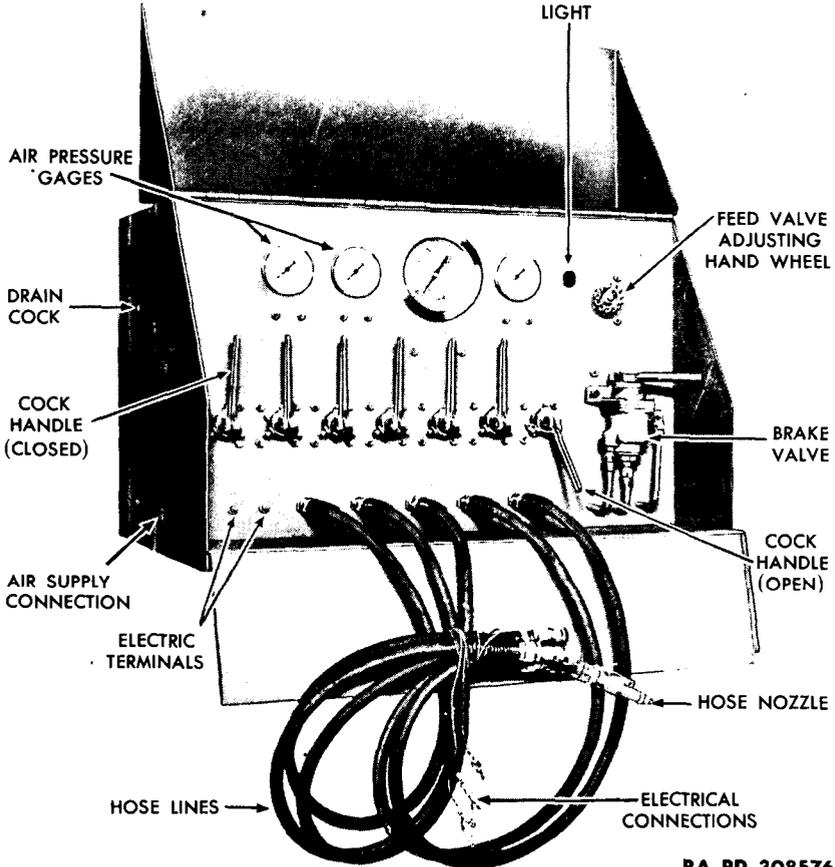
Figure 177 — Portable Test Rack BWE SA-1561-23
