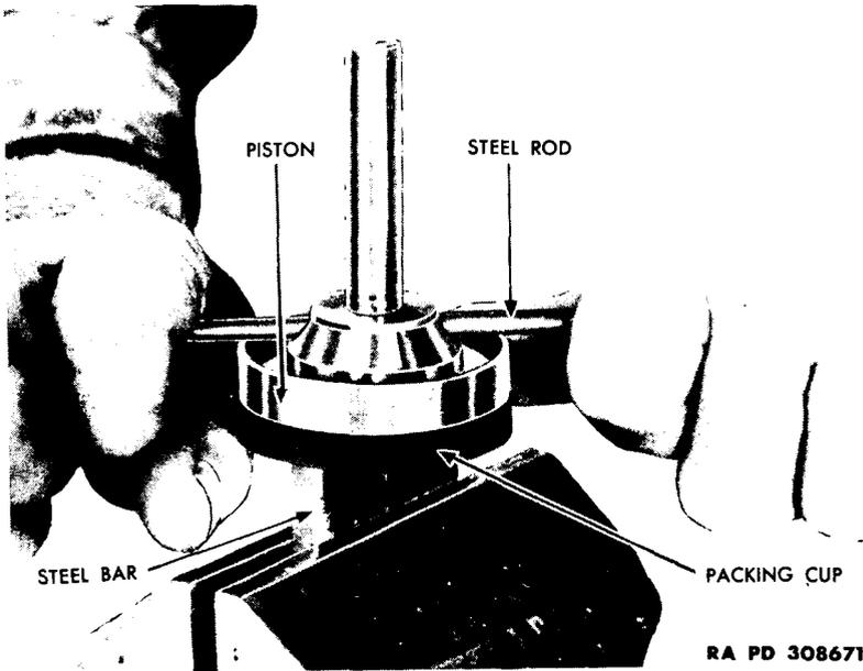
**Figure 66 – Disassembly of Piston**
