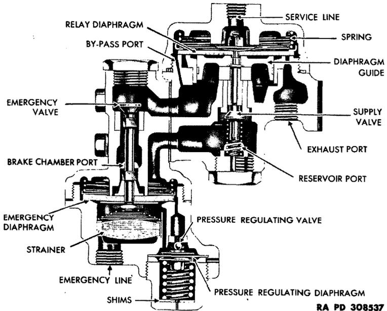
**Figure 95 – Sectional View of Relay Emergency Valve with
