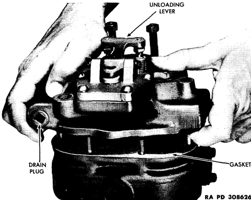
**Figure 12 – Removing Cylinder Head**
