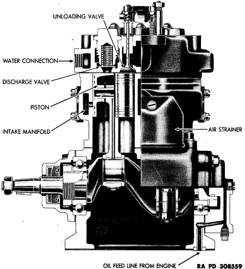
**Figure 8 – Sectional View of a Two-cylinder Engine-lubricated Compressor**
