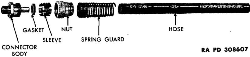
**Figure 129 – Hose Assembly Disassembled**
