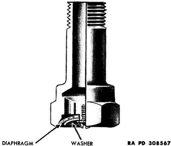
**Figure 121 – Sectional View of Exhaust Check Valve**
