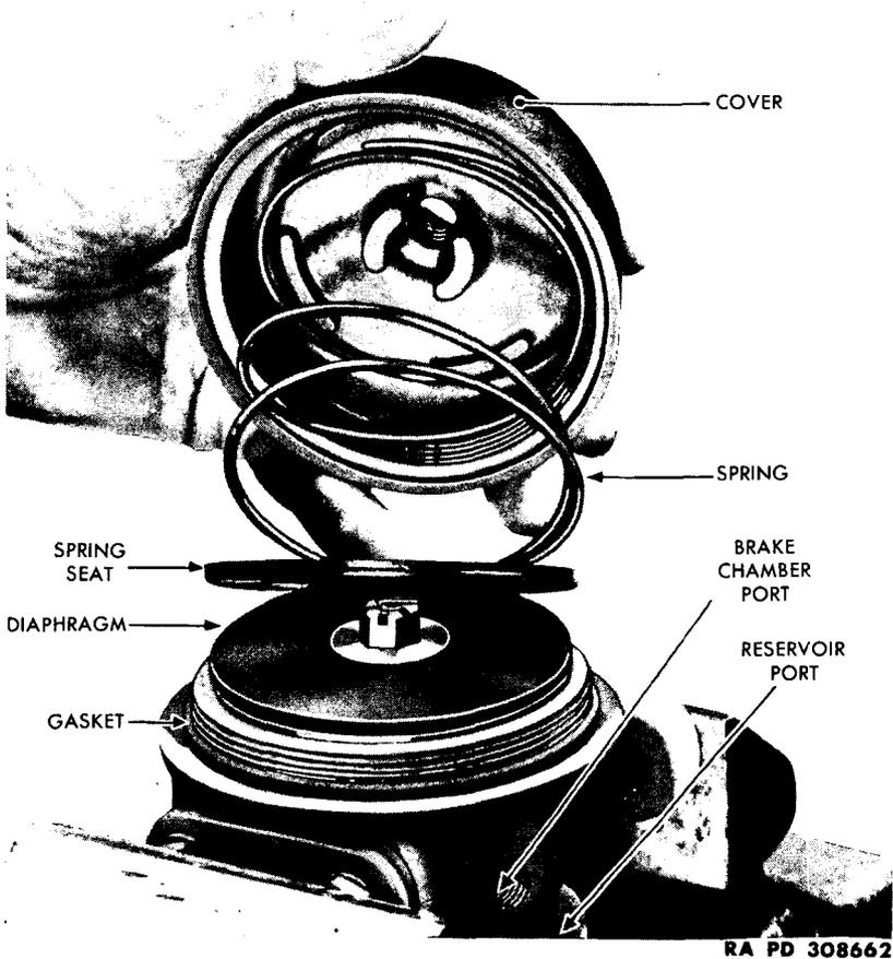
**Figure 84 — Removing Cover**
