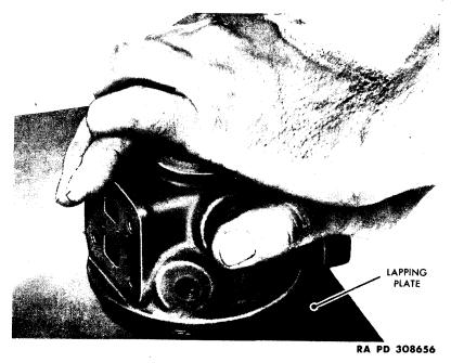
Figure 87 — Lapping Diaphragm Seat
