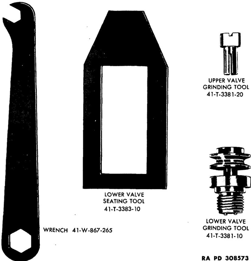
**Figure 168 — Special Tools for Repairing Governors**
