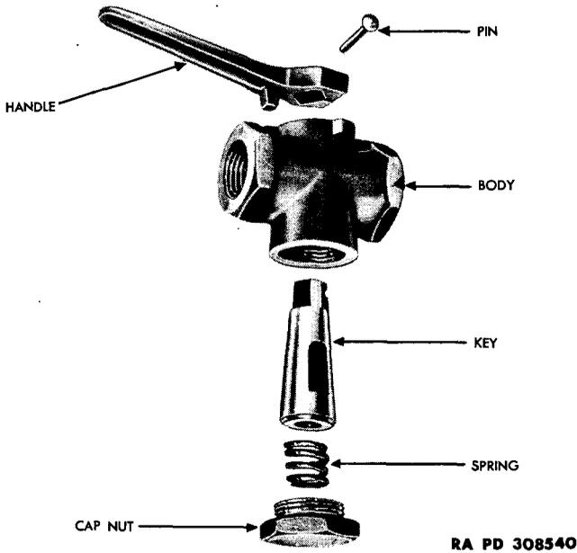
Figure 124 — Cut-out Cock Disassembled
