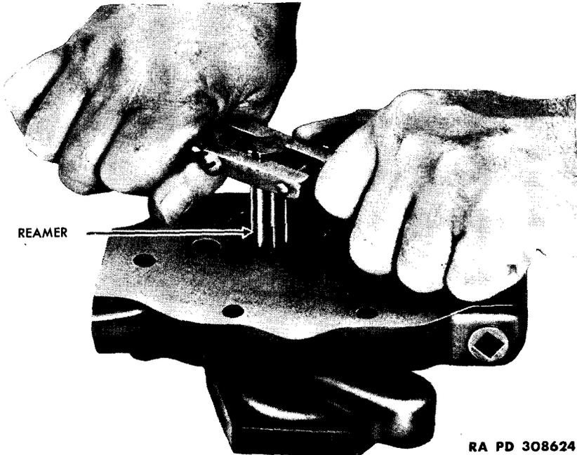
**Figure 22 — Reaming Unloading Valve Seats, Using Reamer 41-R-2309**
