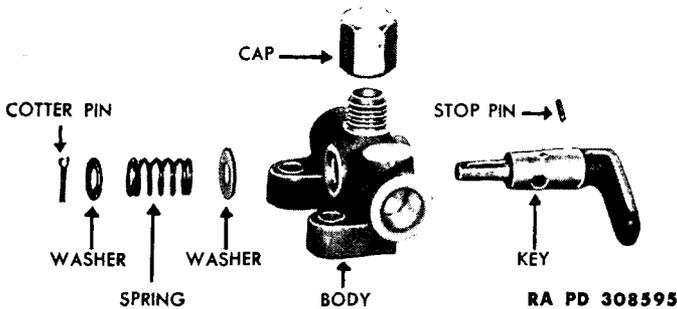
**Figure 158 - Air Supply Valve Disassembled**
